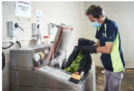
The trial of waste digesters at Sentosa. Photo Credit: SDC
